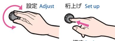
The jog dial is used for output current and voltage setup. One dial is capable of digit-by-digit numerical value setup and moving through values, which allows easy setup.
